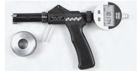
Triga-Bore handle shown with True-Bore Head, Digital Indicator, and Master Setting Ring.
