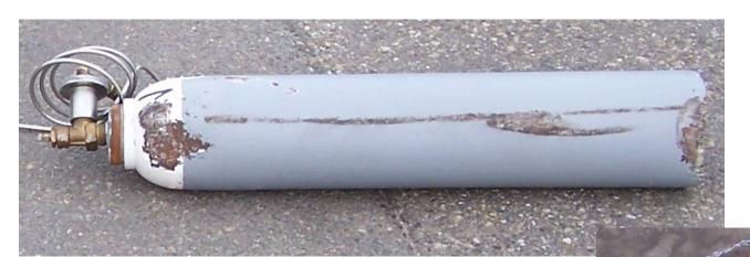
Originally 13.4 litre CO2 cylinder, base cut, barrel shortened and base welded to barrel to look like a 10 litre cylinder
