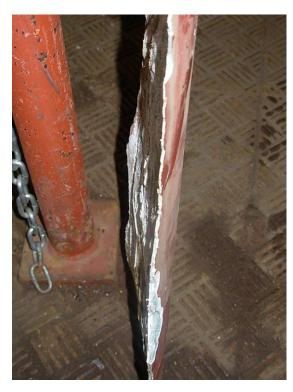
Damaged acetylene cylinder "repaired" with plaster
