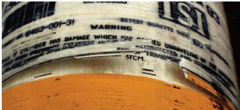
Level 3 delamination—This cylinder must be rejected.
