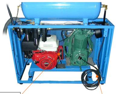
Electric Start with 18 amp Charging Circuit
