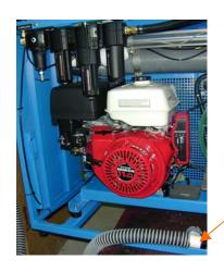
Over Pressure Relief. On end of permeate hose that gets attached to the high or low pressure compressor that will pump the nitrox.
