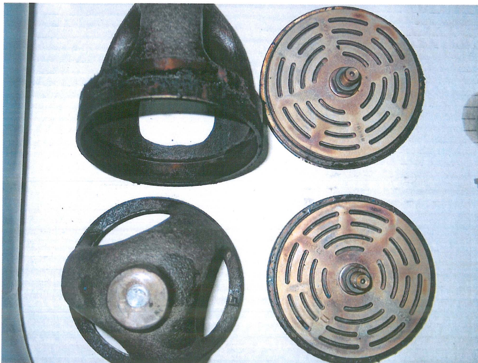
discharge valves IK28.0 1 st stage after 2000 operating hours
