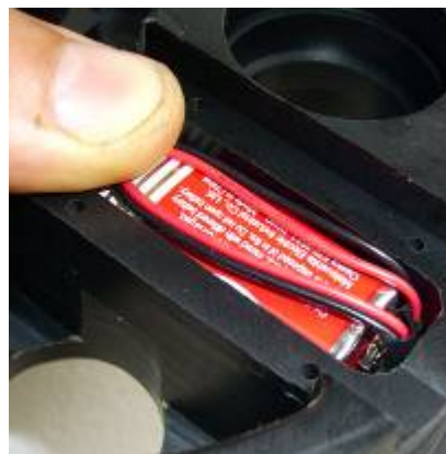
Fig. 8 Long strap, means negative up
