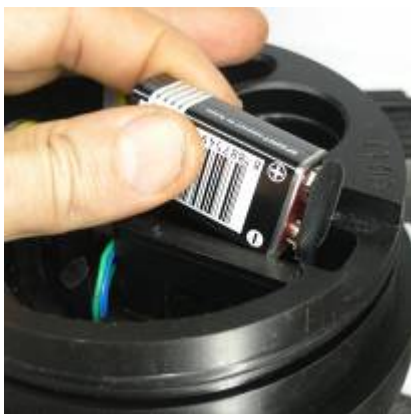
Fig. 7 Short strap, means positive up
