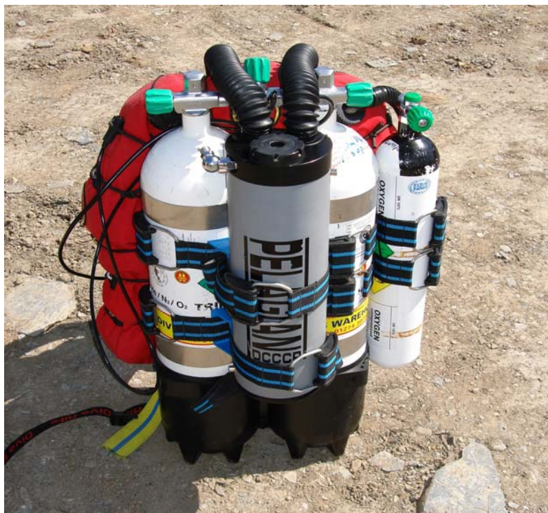
Pelagian Unit used on 150metre dives during an Expedition to HMS Victoria in Lebanon. Scrubber is attached directly to Diluent / Bail-out twinset alongside 5litre oxygen cylinder. Additional decompression tanks worn for open-circuit bail-out decompression.
