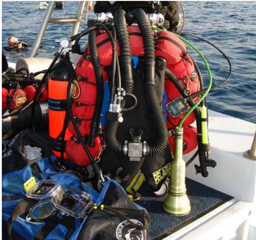
Pelagian Unit used on 150metre dives during an Expedition to HMS Victoria in Lebanon. Scrubber is attached directly to Diluent / Bail-out twinset alongside 5litre oxygen cylinder. Additional decompression tanks worn for open-circuit bail-out decompression.
