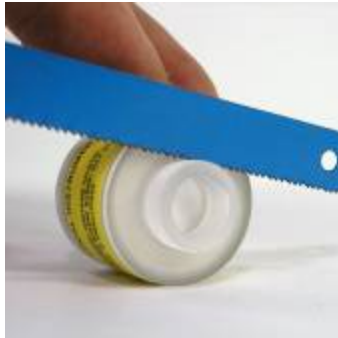
Fig. 1 Cut the threads on all cells rear cut
