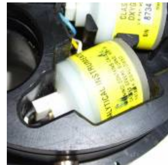
Fig. 6 Cell one in socket
